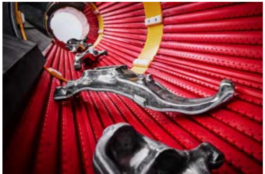
While passing through the trough the work pieces are continuously rotating. This ensures that the blast media is reaching all work piece surface areas, and always from the same distance.
