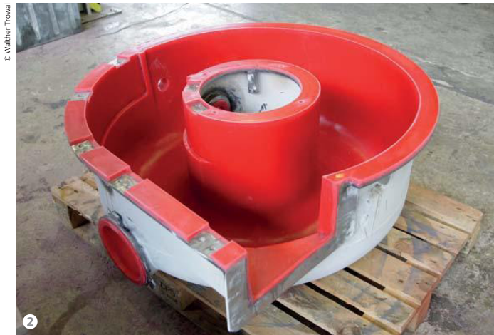
Figure 2: A relined work bowl prior to painting.
