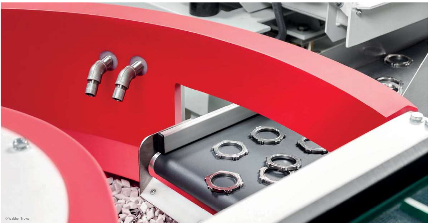
The work pieces are transferred into the machine from the side with a conveyor belt.
