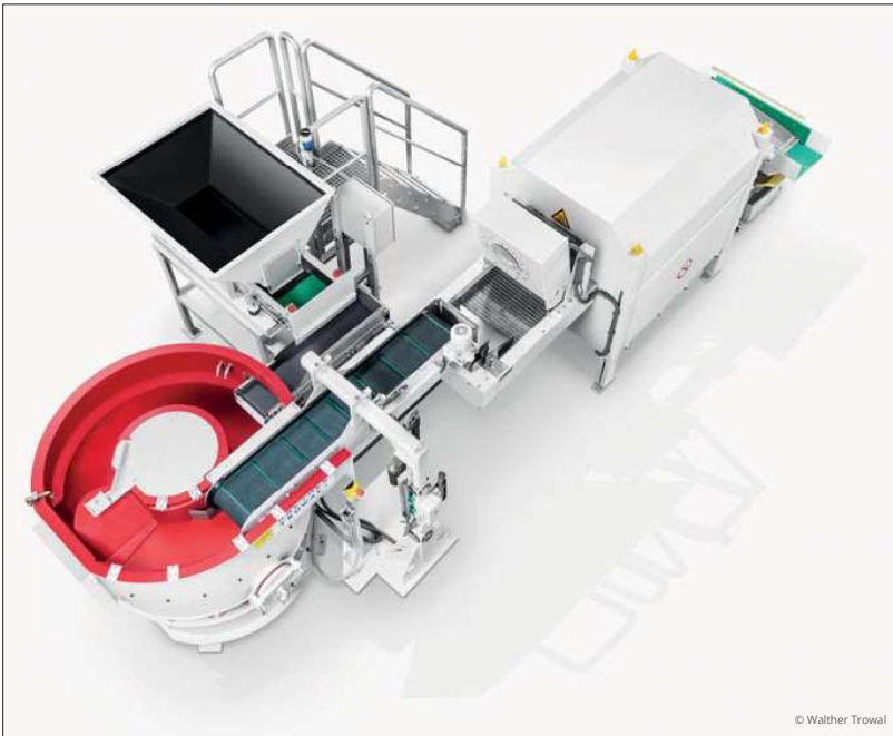
A CB rotary vibrator equipped with a magnetic separator that removes ferromagnetic work pieces from the media mix and feeds them into a drier (visible on the right side of the photo).
