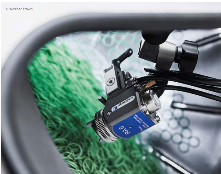
The automatic spray guns are evenly applying the coating material on the surface of the elastomer components.
