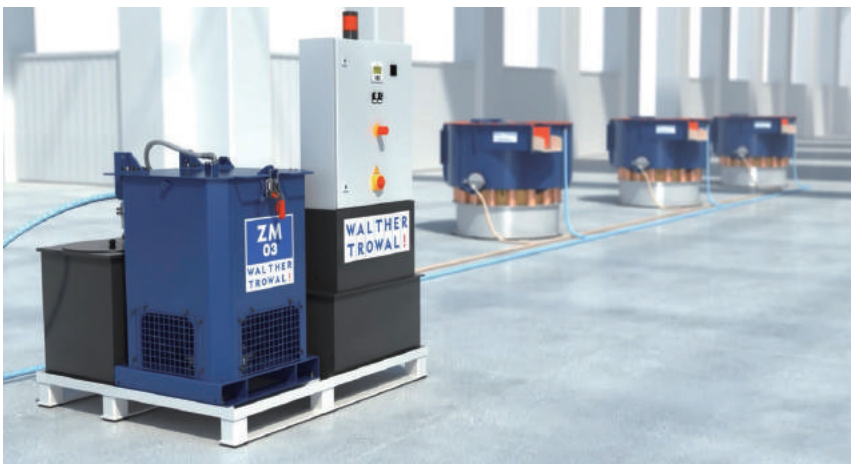
In process water cleaning and recycling systems the contaminants in the form of solids and, sometimes, oil are removed by centrifuges. The cleaned process water does not have to go to drain but can be re-used in the mass finishing process
