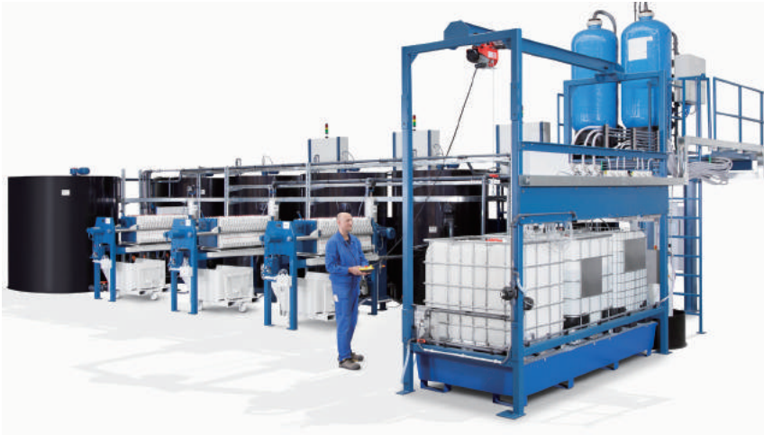
In flow-through systems the contaminated process water is cleaned by flocculation and filtration and then, by being sent to drain, is returned to the pool of fresh water
