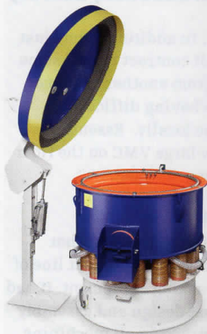
The entire work bowl of the CM vibratory system vibrates to remove burrs and provide a smooth, even surface on blisks.
