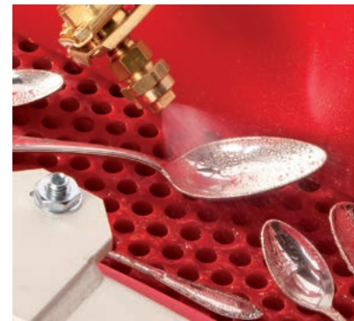
The rinse phase of the cutlery cleaning process
