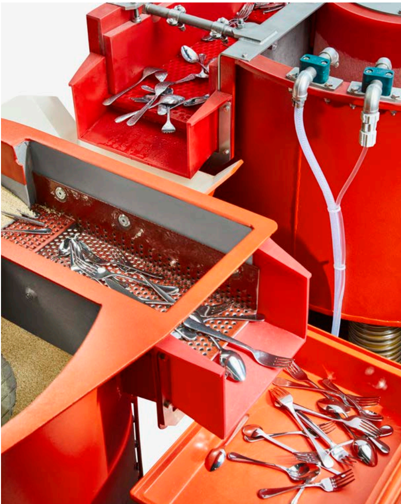
Transfer of the cutlery pieces from the processing bowl into the drier.
