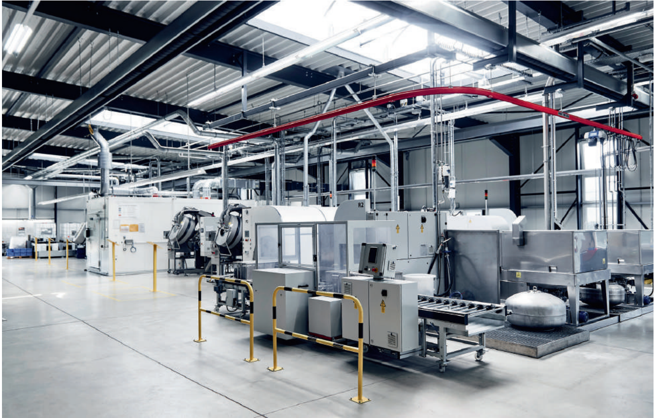
Ten drum coating machines are in use in the new factory building.
