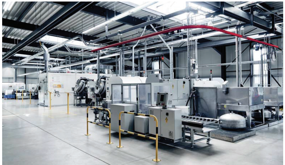
The new production facility is equipped with ten Rotamat coaters from Walther Trowal.
