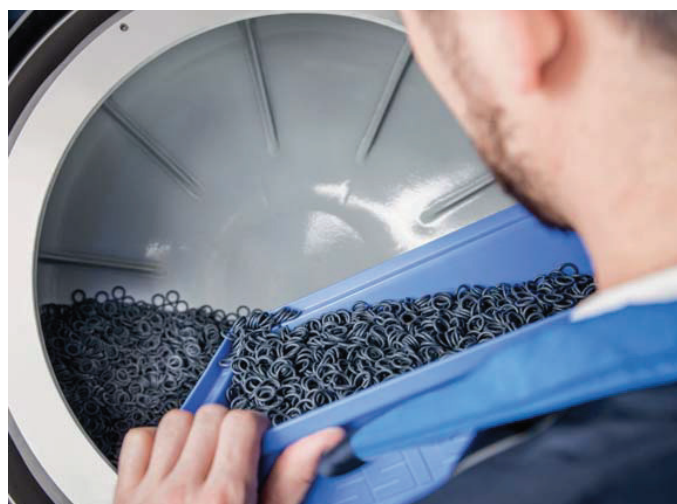
The Rotamat is ideal for coating of mass-produced small parts, for example, made from elastomers (photo) or metal.
