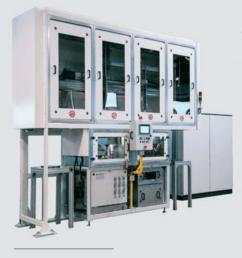
TRIPLE MACHINE, WITH 3 MAGNETIC ARMS AND 3 SPRAYGUNS FOR PAINTING INNER AREA OF METALLIC OBJECTS.
