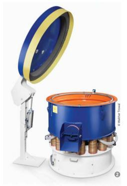
Figure 2: In the "CM" rotary vibrator work pieces with a diameter of up to 980 mm can be processed. During the finishing process itself the work bowl is covered with a noise absorbing lid.
