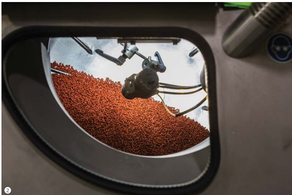
Figure 2: The automatic spray gun evenly applies the coating material onto the gently tumbling mass-produced small parts.
