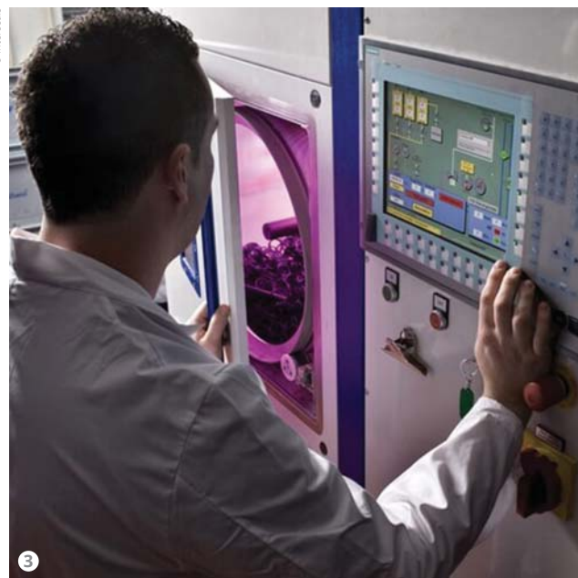
Figure 3: The entire coating process is controlled and monitored by an industrial PC with touch panel integrated into the control panel.
